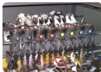
Ink supply and nozzle cleaning system
