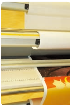
Film and liner separate
