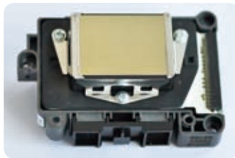
Piezo electric inkjet print head
