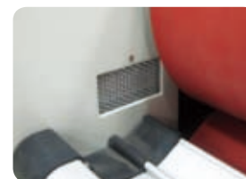
The baffle - board of photocell safety switch
