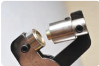
Magnetic dies fix the eyelet and washer well
