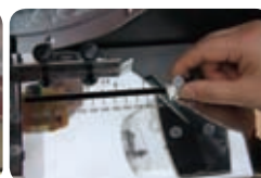
Adjust the spacing and margin of grommet
